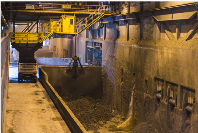
IBA pit at Tuas South Incineration Plant. The NEA is studying the use of IBA for non-structural applications
